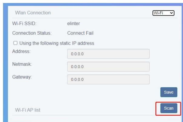
Fig 1.9 Scan WiFi AP list on device web.
