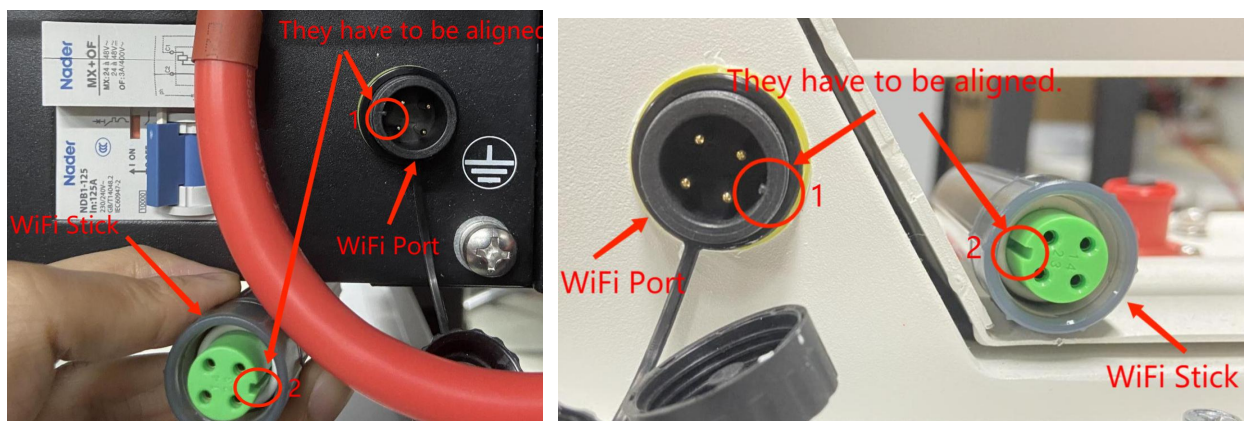
Fig 1.4 Connect WiFi stick to the WiFi port on battery.
