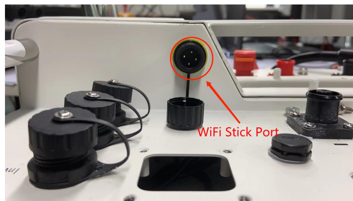
Fig 1.3 WiFi port on PLPA battery.
